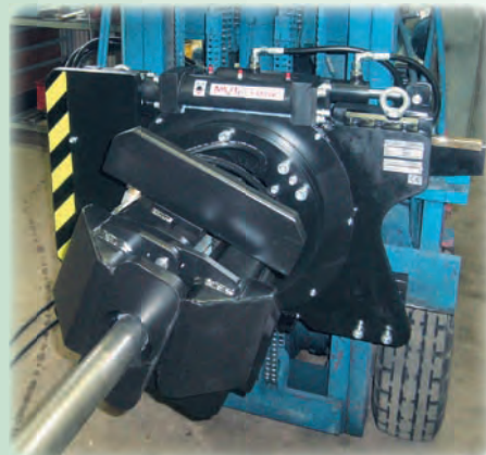
Otoč s uchopovacími čelistmi RA16S-CPT Revolving machine with gripping jaws RA16S-CPT
