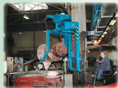
Manipulátor pro manipulaci s kelímkami RSG10M Manipulator for crucibles handling RSG10M
